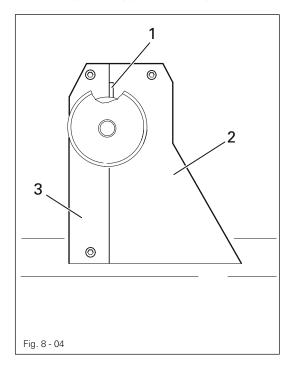
If a large balance wheel is used, the corner **1** of the belt guard **2** must be broken out.
